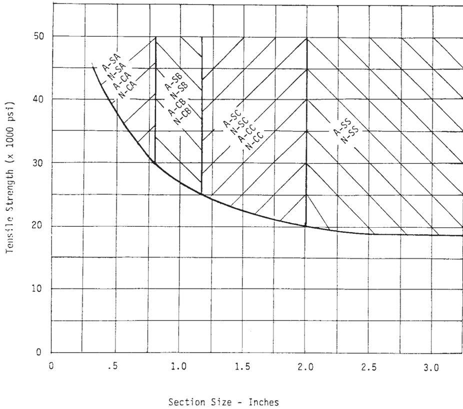
NOTE—The relationship of permanent mold gray iron tensile strength versus section size is shown above. Castings with controlling section up to 0.875 in. will have a minimum tensile strength of 30 000 psi (207 MPa). Castings with controlling section between 0.875 and 1.2 in. will have a minimum tensile strength of 25 000 psi (172 MPa). Castings with controlling section between 1.2 and 2.0 in. will have a minimum tensile strength of 20 000 psi (138 MPa).
